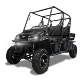
AMP CREW - 4x2 **48V CD LITHIUM-ION** 5KW/8KW 600 amp controller **30MPH** 1,500 lbs 400 lbs
