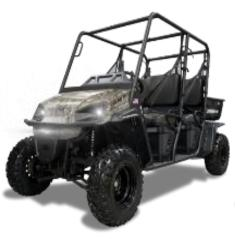
AMP CREW - 4x4 **48V CD LITHIUM-ION** 8KW 600 amp controller **30MPH** 1,500 lbs 400 lbs
