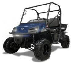
AMP - 4x4**48V CD LITHIUM-ION** 5KW/8KW 600 amp controller **30MPH** 1,500 lbs 600 lbs
